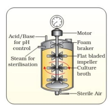
(iii) The stirrer facilitates even mixing and oxygen availability throughout simplestirred tank bioreactor, whereas in case of sparged stirred-tank bioreactor, air is bubbled throughout the reactor for proper mixing.
